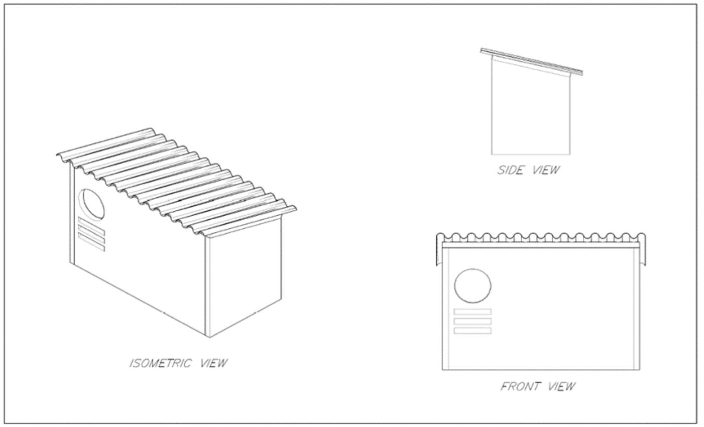
Barn Owl Boxes are mounted on a two ½-inch steel pole, and should be approximately 8 feet above the ground to prevent predators from entering which includes Great Horned Owls, raccoons and hawks. Boxes should be installed facing Northeast, which allows the least amount of light in and offers the best protection from the wind.
