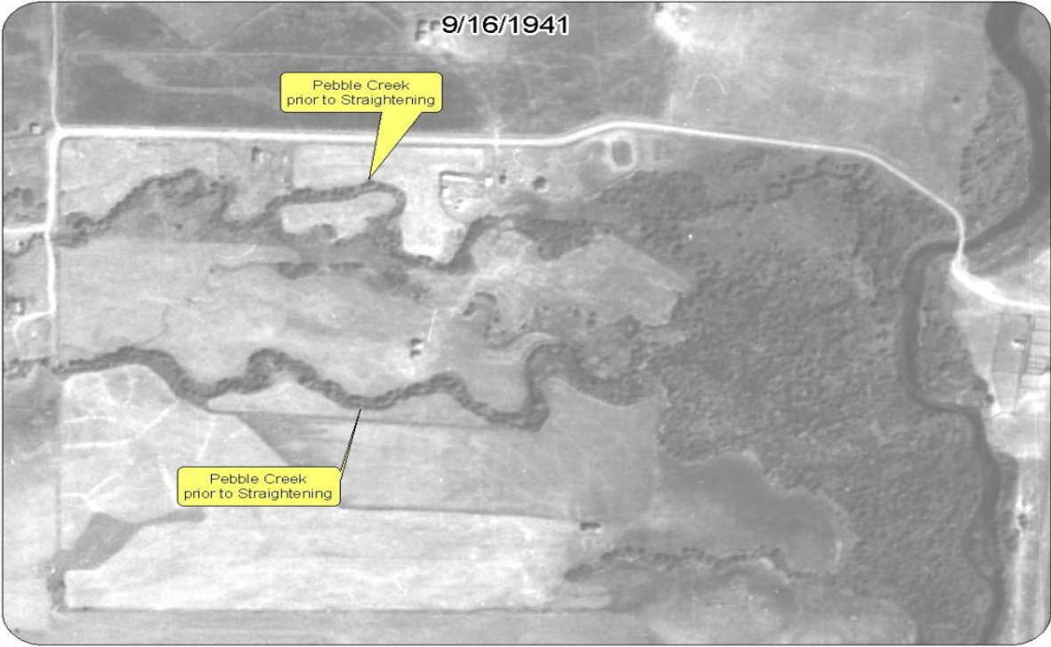
Photo 1-This photo was used as the basis for the new channels to be designed, Pebble Creek Restoration.
